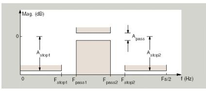
In this example, a sampling frequency of Fs = 48 kHz is used. This bandpass filter has the following specifications, specified here using MATLAB code:
